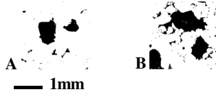
Fig. 7. Pore Type 5. A-B: Very large pores associated to dissolved feldspars.
